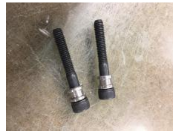
The Bolts with the Clip Fitting installed.
